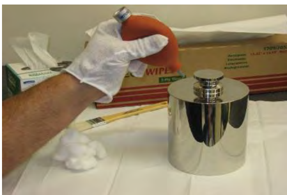
Figure 1.5-6: Cleaning the TI Using an Air Puffer
