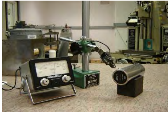
Figure 1.1-16: V-Blocks to measure roundness
