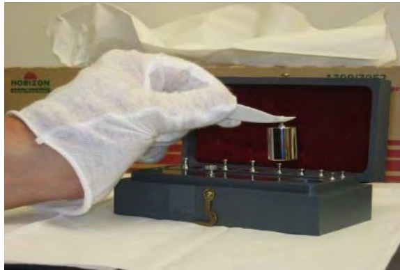
Figure1.5-8: Using forceps to Handle Small Weights
