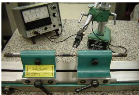
Figure 1.1-14: Bench centers to measure roundness
