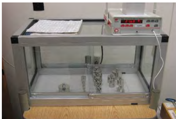
Figure 1.5-4: Mass Standards in an Enclosure
