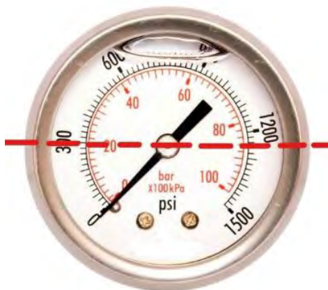
Figure 1.6-11: Dial Gauge Head Height Location
