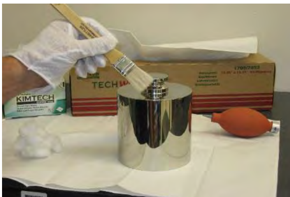
Figure 1.5-5: Cleaning the TI Using a Brush
