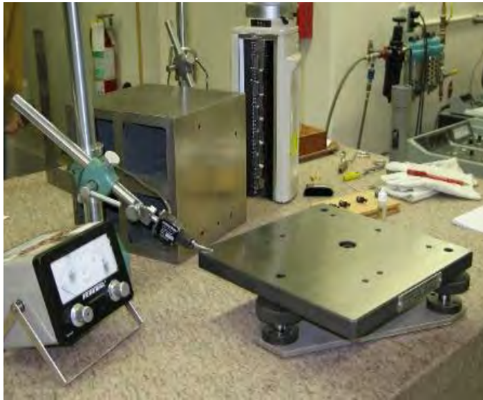
Figure 1.1-2: Electronic Height Gage and Leveling Plate
