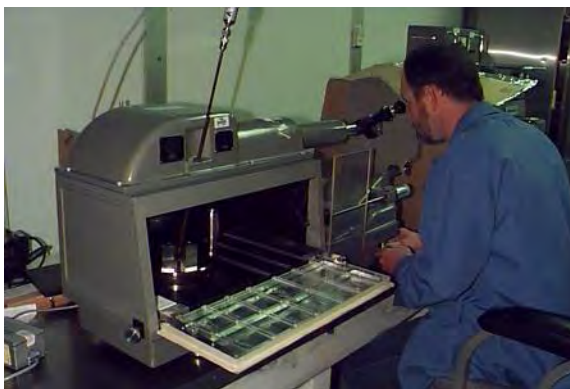
Figure 1.2-3: Interferometric Gage Block Calibration
