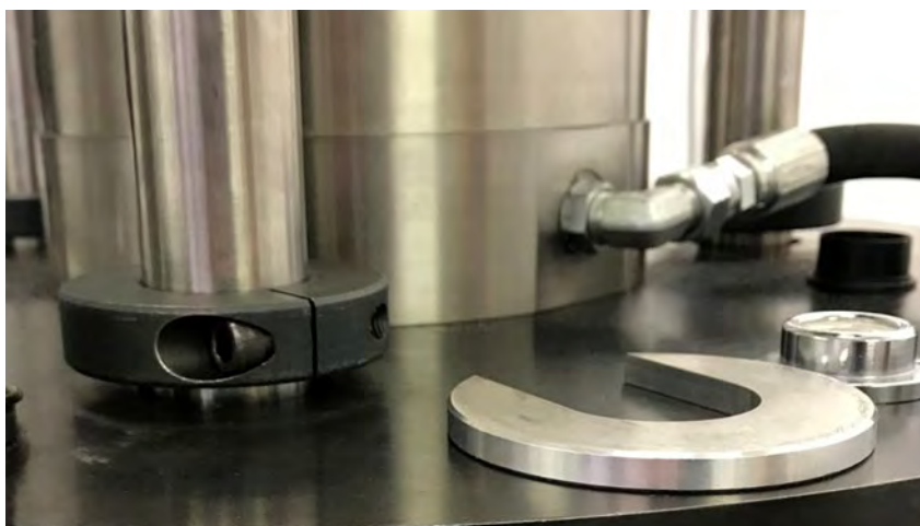
Figure 1.10-3: Vertical Force Press Locking Collar
