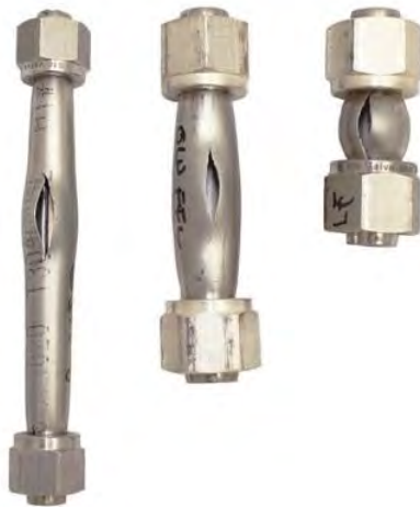
Figure 1.6-10: Tube Failure
