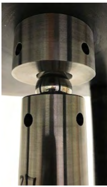
Figure 1.10-5: Compression Ball Centered with Adapter
