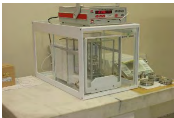
Figure 1.5-3: Balance with Draft Shield and Enclosure
