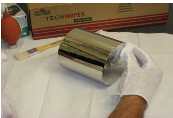
Figure 1.5-7: Cleaning the TI Using a Cotton Ball
